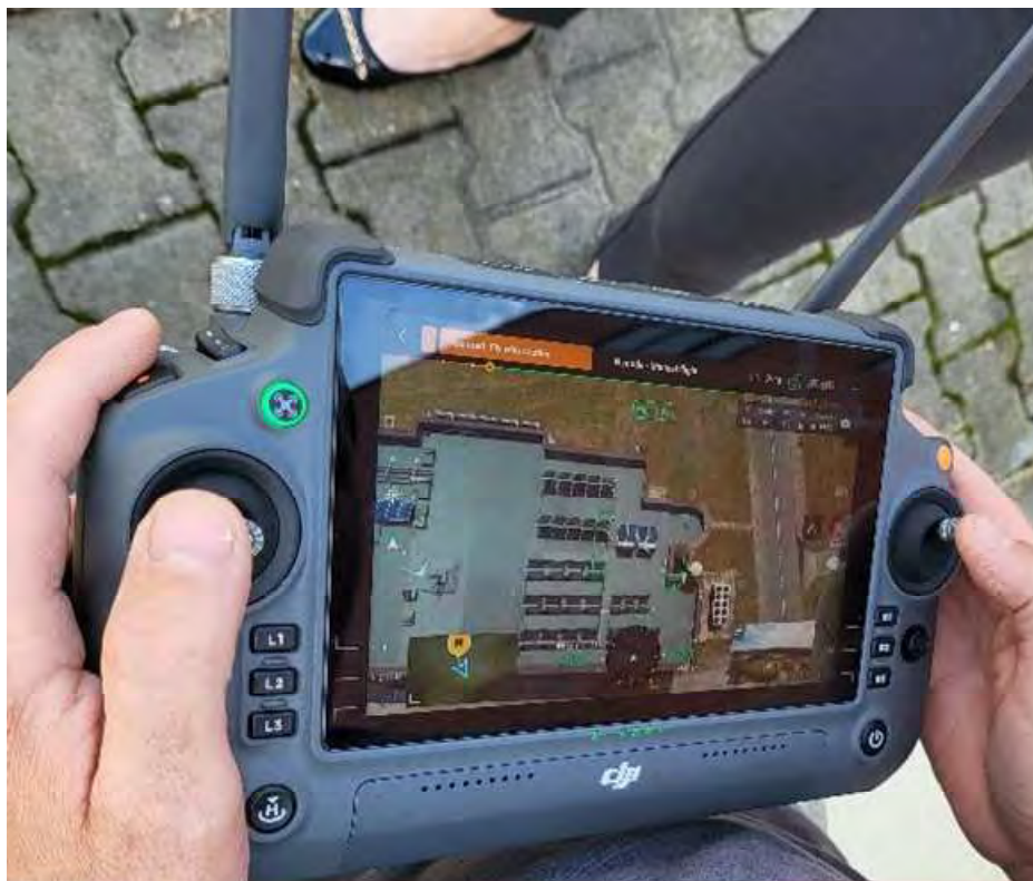
Figure 4.53 – Piloting and collecting thermal data
