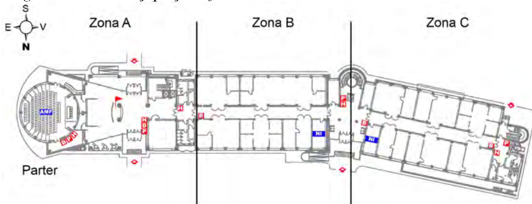
Figura Error! No text of specified style in document..5 - Compartimentarea si zonarea ICSTM
