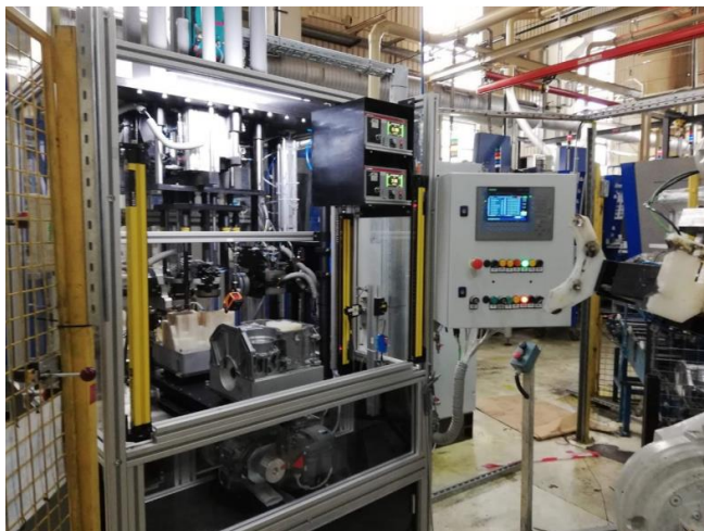
Fig. 15.1 - Ultra-precise cyber-mechatronic industrial and laboratory control system for cast parts from automotive industry (implemented in production line)
