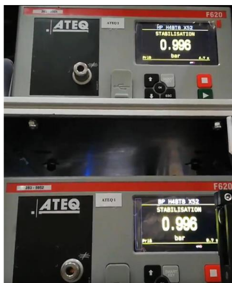
Fig. 14.2 - Stabilization of pressure circuits
