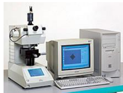
Figure 5. Automatic reading system for Vickers hardness tests
