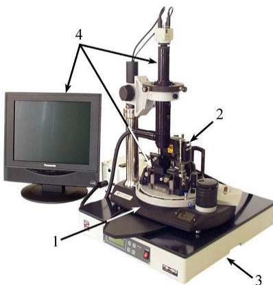
Figura 4. Microscop AFM, NTEGRA Probe NanoLaboratory NT – MDT, Moscova, Rusia.
