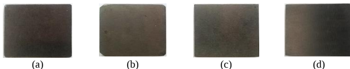
Figure 3. Steel substrates on which nanometric metal layers have been deposited using electron beam evaporation: (a) OLC45; (b) Ru11; (c) C120; (d) CSO
