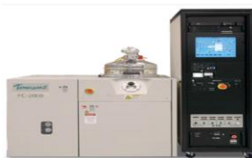
Figure 2. Temescal FC-2000 - electron beam evaporation deposition system.
