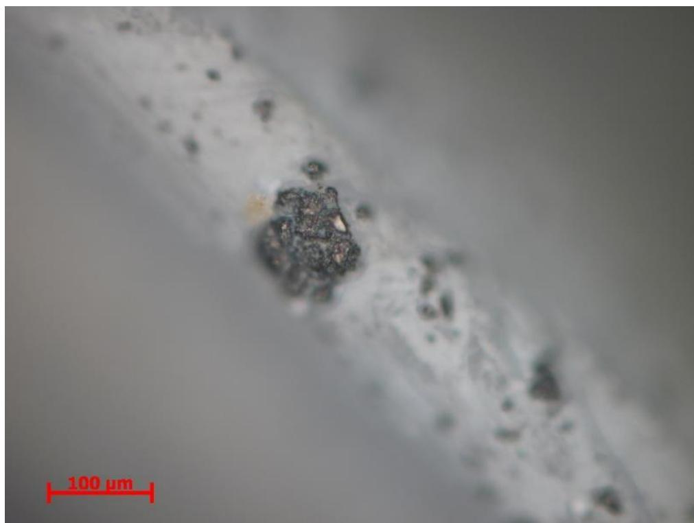
*Figure No. 6.1-optical microscopy of the innovative implant impregnated with carbon nanotubes*
