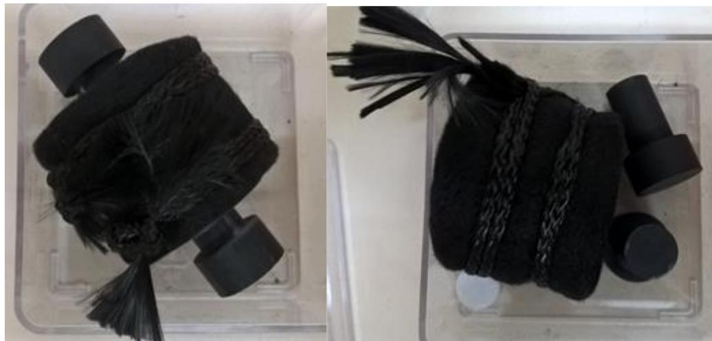
*Figure No. 8.38-Graphite plates for spark plasma sintering system*
