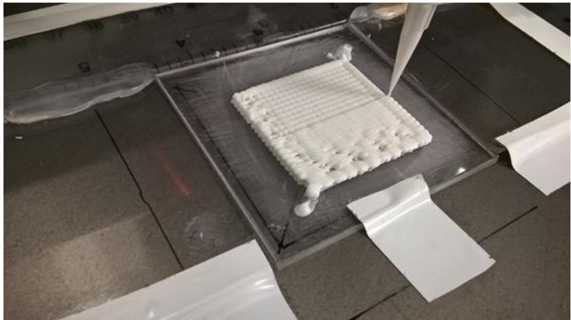
*Figure No. 8.1: Extrusion bioprinting (SYS system + ENG Bioscaffolder-INCD-IMNR Research Laboratory)*
