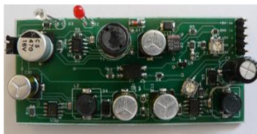
Figure no. 7.5 - Original Circuit of the Power Supply Circuit (PCB) assembly
