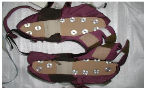
Figure no. 7.2 - Sensor mounting solution applied on the overshoes
