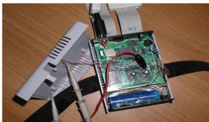
Figure no. 7.6 - Internal view of the Acquisition Unit box with microprocessor
