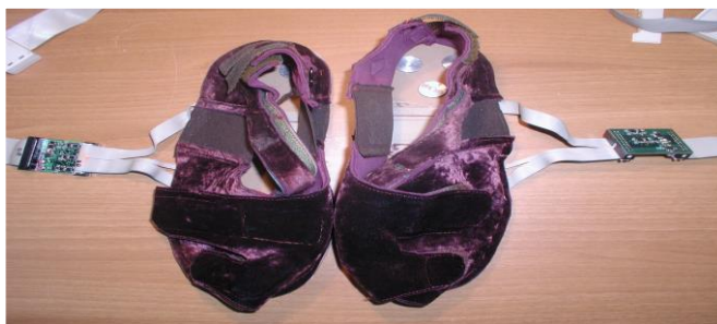
Figure no. 7.8 - Final version of the overshoe support with sensors
